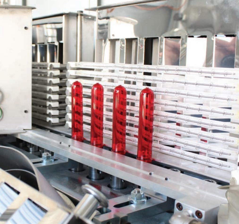
Left: Oven banks receive the preforms. Above and below: High-precision blow moulding
